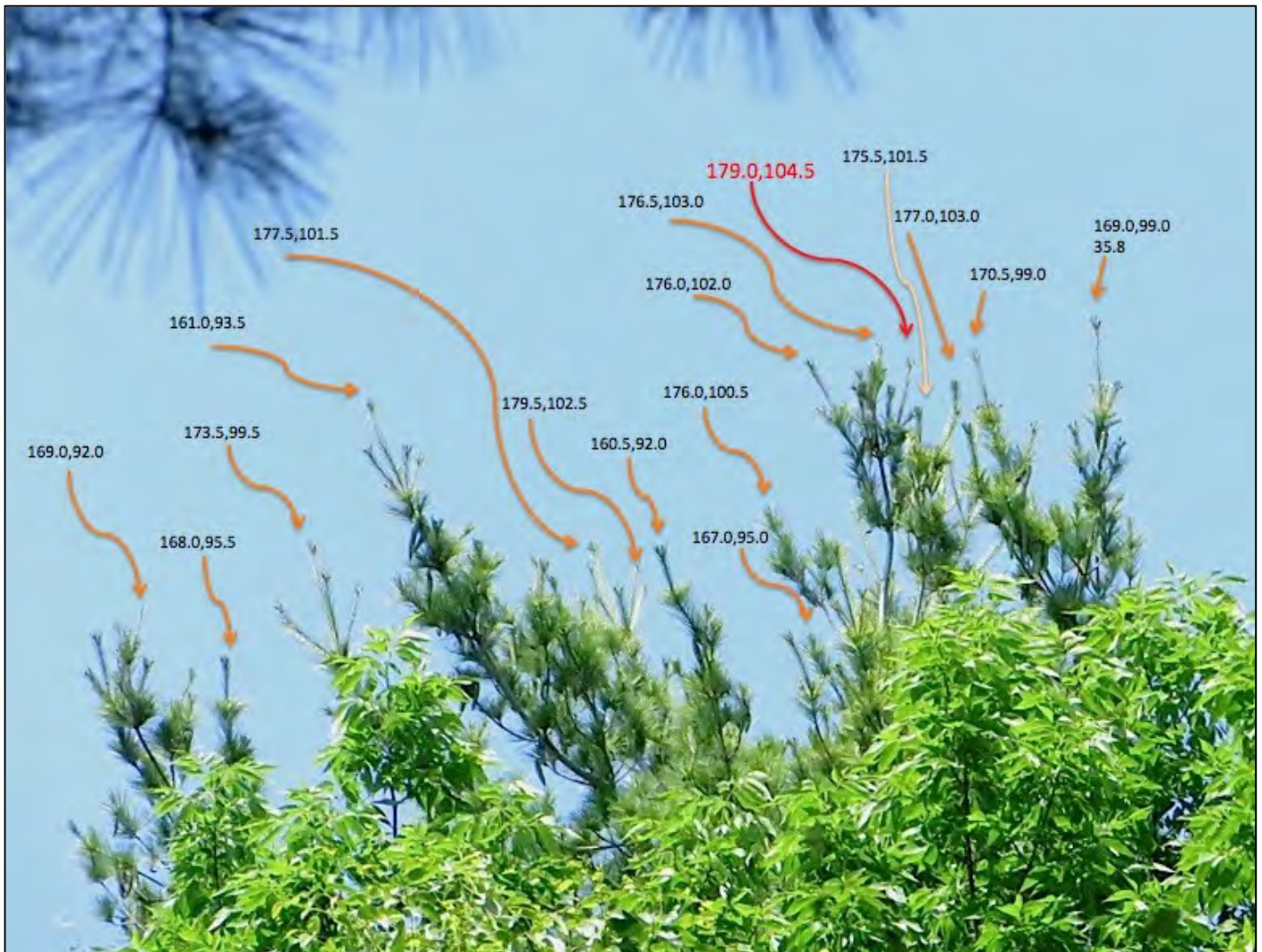
Figure 2. Different slope distances (first number) and vertical distances (second number) for the various leaders of the Monica Pine. The number highlighted in red is the highest vertical height value from this vantage point.
