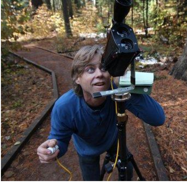
measuring the 253'+ sugar pine with Impulse200LR laser and prism/pole survey
