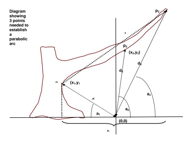
$I_1$ =slope distance between  $p_1$  and  $p_3$  $h_1$ =horizontal offset distance between  $p_1$  and  $p_3$
